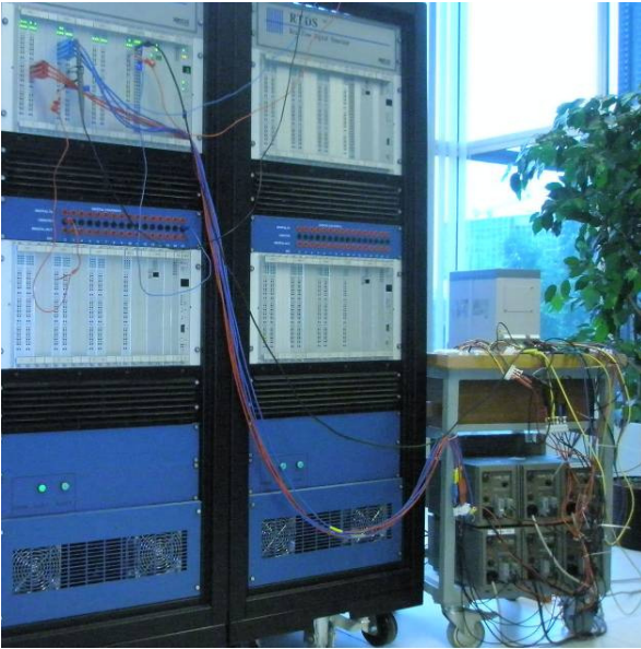
Fig. 7. Closed-loop relay test circuit.
